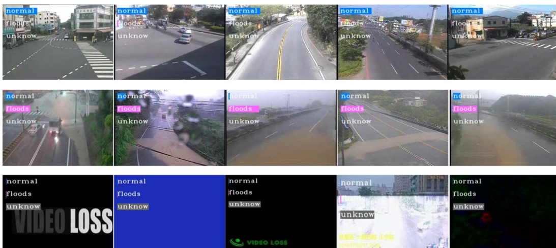
FIGURE 5. Example of the scene recognition result from the model. The top, middle, and bottom rows show the results for the normal, flood, and unknown scenes, respectively. The label bars represent the confidence scores for each class (in percentage points).
