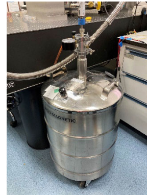
FIGURE 3. LN-50 liquid nitrogen dewar developed by Janis, an American company.
