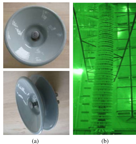
FIGURE 1. Insulator monolithic sample and long string experiment diagram. (a) Single piece double umbrella sample insulator. (b) Long string insulator experiment diagram.
