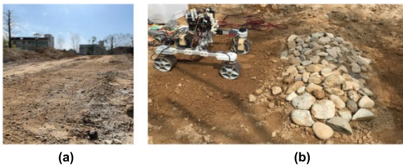
FIGURE 22. Field test operational environment on (a) terrain approximately inclined at 17° and (b) 0.22-m rocky obstacle under soft soil.
