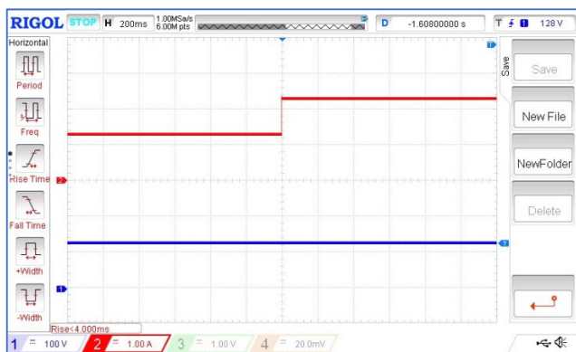
FIGURE 33. Effect of load change from 100\Omega to 54.45\Omega ohm at V_{in} = 15 V on V_o .
