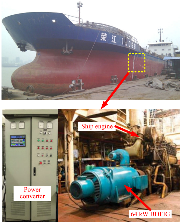
FIGURE 4. The BDFIG application in ship shaft power generation [12].
