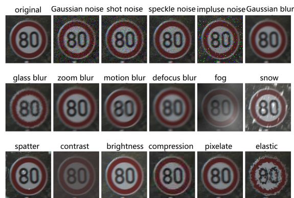
FIGURE 11. The original image with the generated images by 17 different corruption methods.
