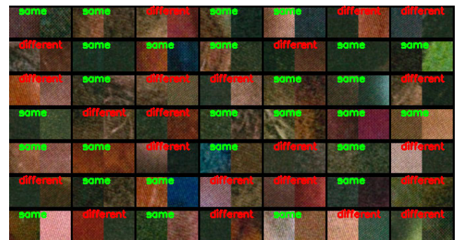
FIGURE 6. Some examples of top energy image patches coming from different (in green) and the same printer (in red). From the figure, it can be noticed that the SNNs learn specific printer artifacts for verification regardless of whether the patterns in the pair are similar or not.
