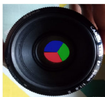
FIGURE 1. Red, green and blue filters arrangement as aperture.
