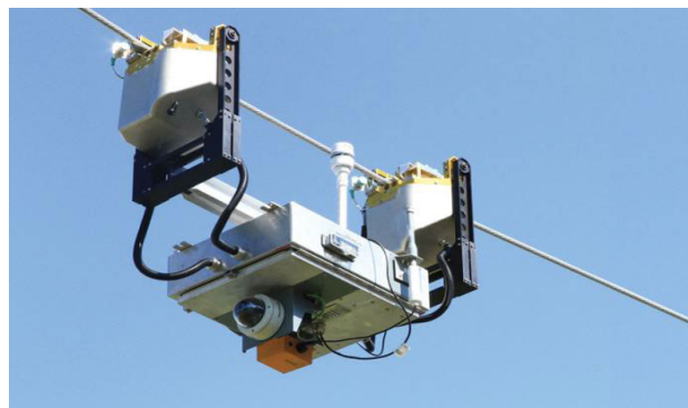
(b) CIR climbing robot is walking through ground wire.
