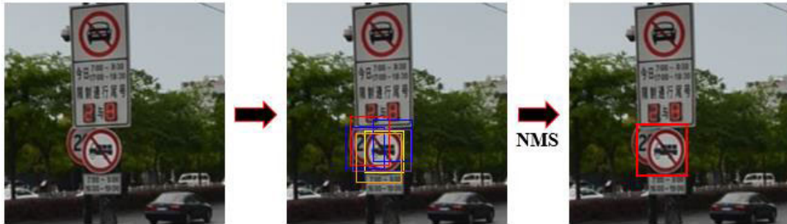
FIGURE 4. Schematic diagram of missed targets in NMS algorithm detection.
