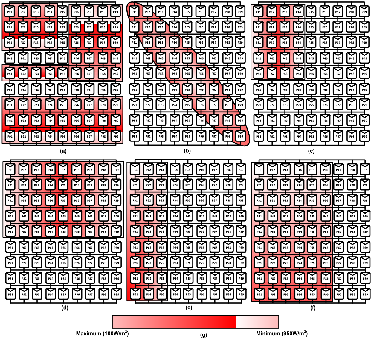
FIGURE 8. Shading patterns (a) Random shading (b) Diagonal shading (c) Short and narrow shading (d) Short and wide shading (e) Long and narrow shading (f) Long and wide shading.
