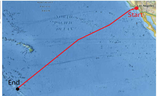
(b) The first real-life existing submarine cable path (Cable SX) drawn using ArcGIS.
