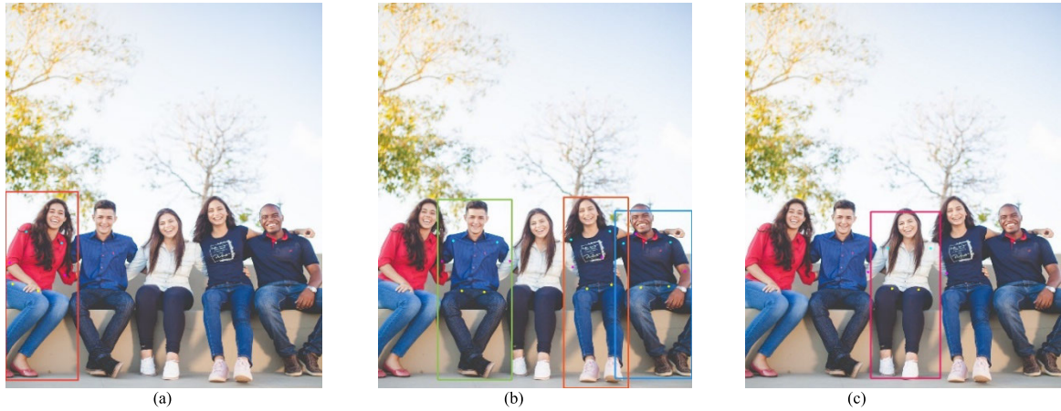
FIGURE 6. Visual evaluation on the same image. (a) To detect red top, (b) To detect blue top, and (c) To detect white top.
