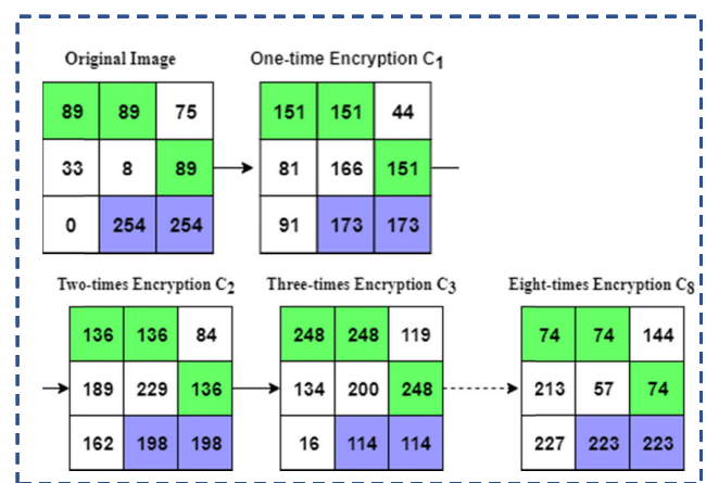
FIGURE 2. High correlation and deterministic problems in multiple-times S-box encryption ( n = 8 ).
