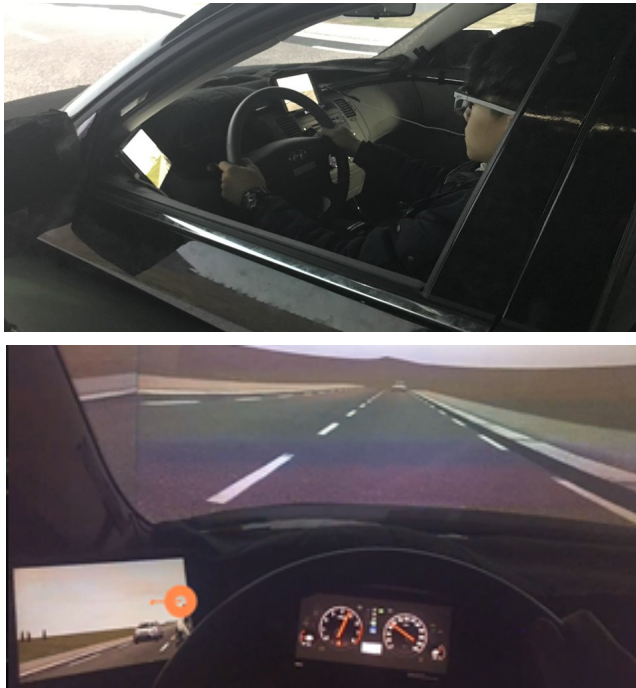
FIGURE 1. Experiment environment with E-mirrors positioned near the sides of the steering wheel (ML 2 ) (top panel) and driving scene taken by the eye-tracking device (orange circle indicates the gaze fixation of a driver; bottom panel).
