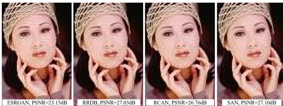
FIGURE 10. SR images produced by various SRDNN methods when the LR image was compressed (JPEG 80). The SRDNN methods were trained using uncompressed LR images.
