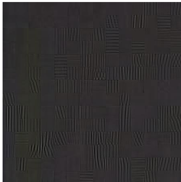
FIGURE 27. Sub-image enlarged by ESRGAN (perceptual). The enhanced coding artefacts (DCT patterns) are clearly visible.
