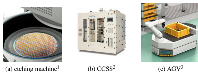
FIGURE 2. The examples by equipment type: (a) A production equipment named etching machine in semiconductor manufacturing creates chip features by selectively removing dielectric and metal materials on a wafer; (b) An infrastructure facility called the central chemical supply system safely supplies high-purity chemicals to the semiconductor manufacturing process; and (c) A logistics automation equipment called automated guided vehicle transports product components in work areas.
