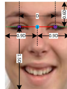
FIGURE 4. Systematic representation of step used for face cropping on a sample facial image from the RaF dataset.
