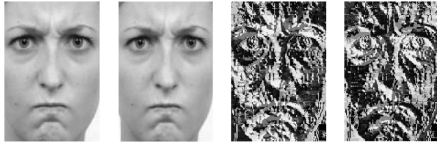
FIGURE 8. Results of global contrast normalization image pre-processing operation (left to right): Original image, GCN enhanced image, DLTP encoded lower image, and DLTP encoded upper image.
