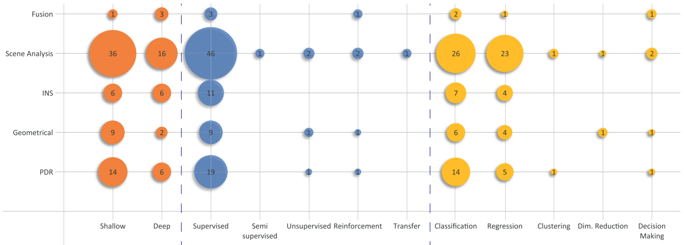
FIGURE 6. ML application in pedestrian localization techniques. The value shown corresponds to a percentage that is calculated based on the 130 papers considered in the systematic literature review.
