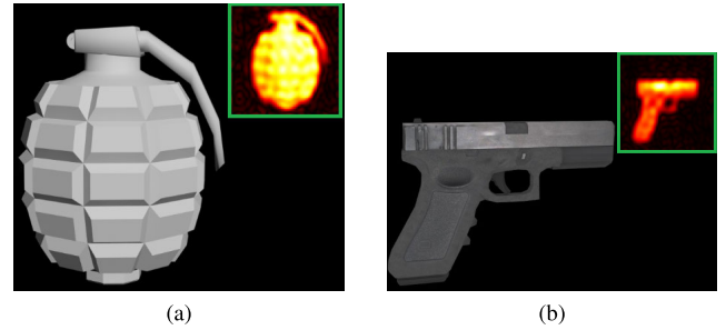
FIGURE 3. Images of two classes of threat objects (a) 2D CAD model of a grenade and CI reconstructed mmW image shown as inset (b) 2D CAD model of a gun phantom and CI reconstructed mmW image shown as inset.
