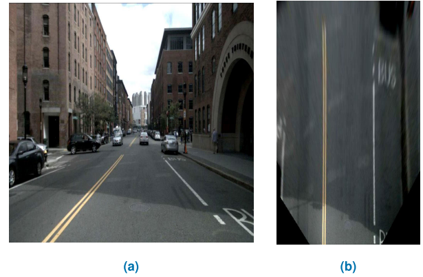
FIGURE 6. Applying perspective transform: (a) The normal scene view; (b) Result of perspective transform.
