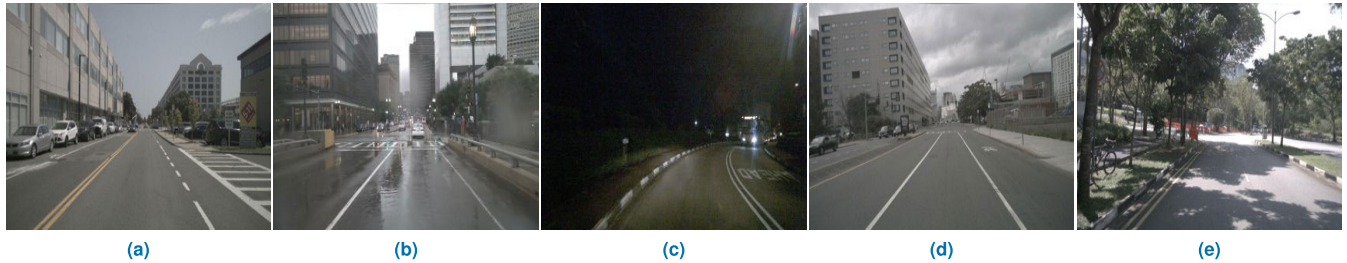
FIGURE 9. A sample from the selected frames of nuScenes dataset: Frame (a) is at daylight; (b) is rainy; (c) is at night, (d) is cloudy, and (e) is shadowy. Frames (a) and (e) contain yellow straight lane lines; (c) contains curved white lane lines; while (b) and (d) contain white straight lane lines.
