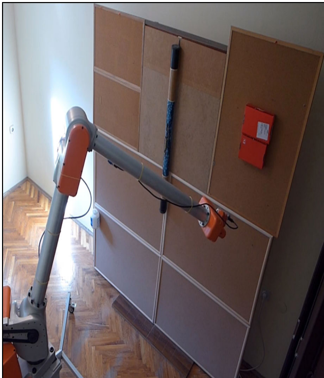
FIGURE 2. The painting robot in the testing process.
