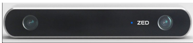
FIGURE 3. The ZED depth sensor.
