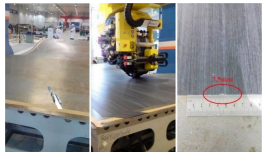
FIGURE 2. Excessive gaps appear at the end of laid tapes.
