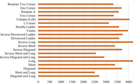
FIGURE 35. Comparison of P_{MP} in Watts for HC configuration with 5 \times 5 array size under each partial shading pattern.
