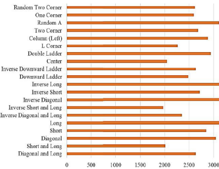
FIGURE 28. Comparison of P_{MP} in Watts for BL configuration with 5 \times 4 array size under each partial shading pattern.
