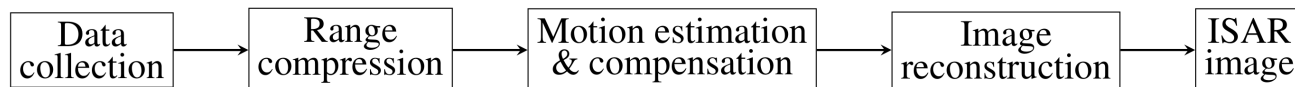
FIGURE 2. Flow chart depicting the conventional ISAR processing chain. Target motion estimation and compensation are prerequisites for successful image reconstruction.
