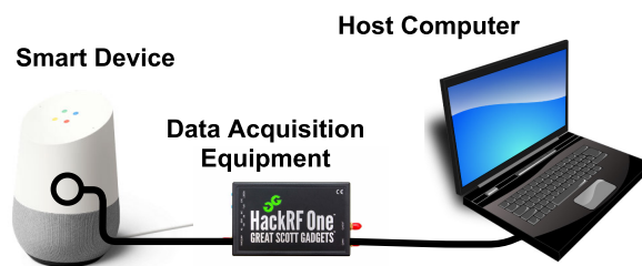
FIGURE 1. The hardware setup for acquiring EM radiation from a smart device. The data acquisition equipment – an SDR in this case – is connected with an H-loop near-field antenna from one end and with a host computer from the other end. Near-field probe is placed over the smart device, i.e., DUT, in order to capture and save EM trace files on the host computer.
