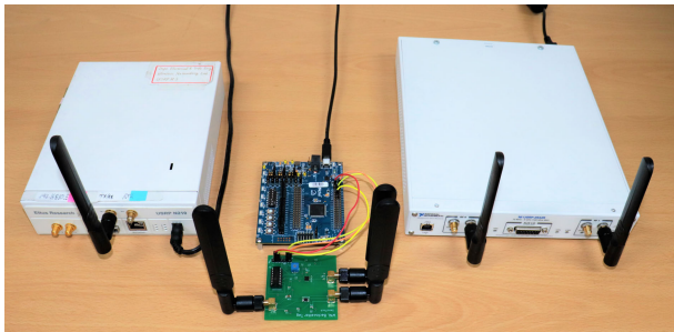
FIGURE 7. Tag hardware prototype and testbed configuration.
