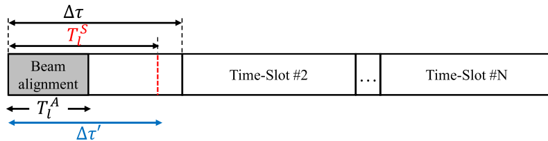
FIGURE 2. Time-slotted communication. Beam alignment can be performed in the beginning of each time-slot if necessary. T_l^S, T_l^A, \Delta\tau' represent link stability time, beam alignment time, and effective time-slot duration, respectively.
