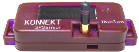
FIGURE 12. Enclosure of the wireless sensor node.
