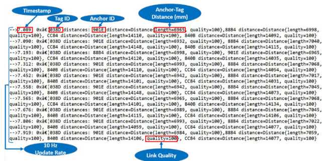
FIGURE 14. An example of the data gathered for test point 1, where the distance between the tag 038D and anchors A08 (840B), A09 (CC84), A15 (8884) and A20 (901B) is shown.
