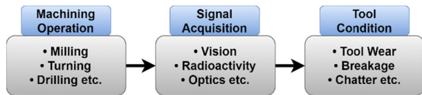
FIGURE 18. Generalized direct tool condition monitoring method.
