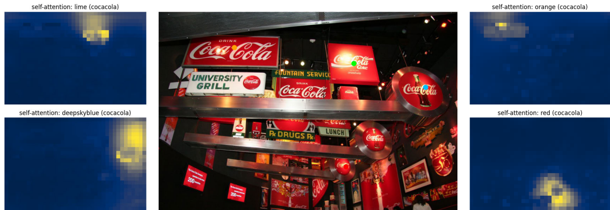
(a) DETR encoder self-attention feature map, visualized around the center of four random ground truth annotations.
