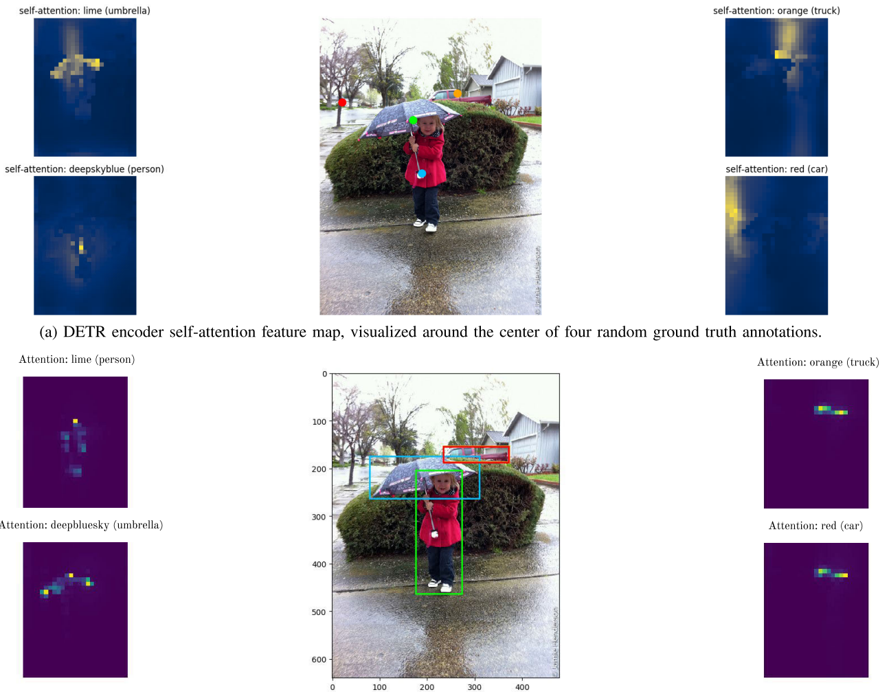
(b) DETR decoder attention map, for the four detections with highest score.
