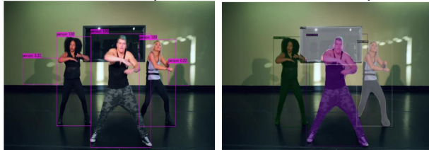
(b) Detectron2 returns higher number of / better objects - here YOLO incorrectly marks the shadows as separate persons, while Detectron2 detects the three persons and the TV correctly.
