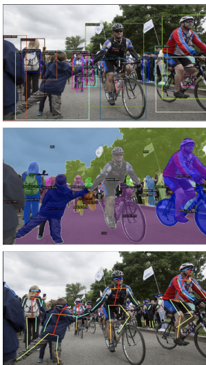
FIGURE 4. Detectron2: (Top) object detection and marking bounding boxes (Center) object segmentation (Bottom) human pose estimation.
