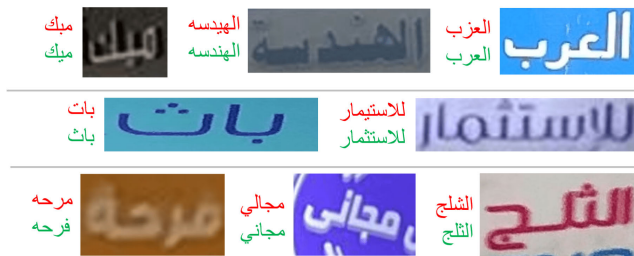
FIGURE 11. Characters misrecognized because of misrecognized dots. Misrecognized word in red and ground truth in green.
