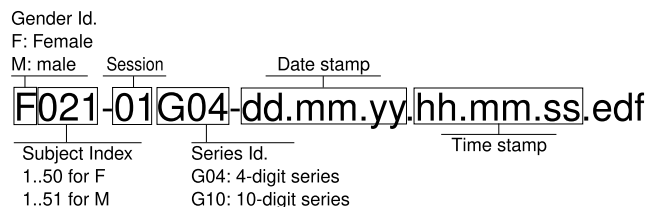
FIGURE 5. Nomenclature configuration for the generated EDF files. G04 files contain the 10 four-digit series, whilst G10 contain the 10 ten-digit ones.
