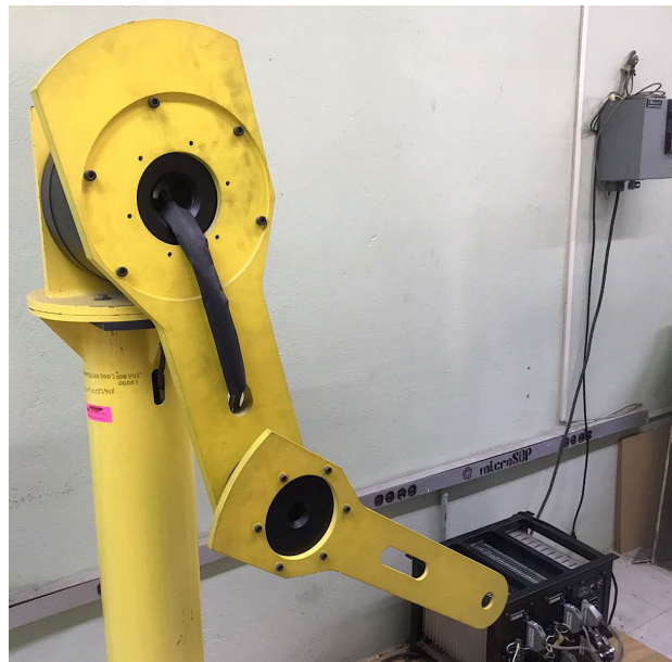
FIGURE 7. Robotic manipulator platform used for the experimental validation. It is a 2-DOF manipulator actuated by direct-drive brushless servo motors operated in torque mode.
