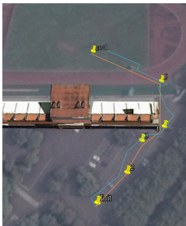
FIGURE 16. The initial path as planned (yellow line) and the actual path recorded by the quadrotor (blue line). The obstacle is bypassed during the flight.
