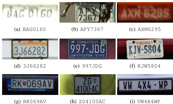
FIGURE 10. Examples of license plates that were correctly recognized by the CNN-OCR architecture. The images in the first row belong to our dataset while the others belong to public datasets acquired in other countries.
