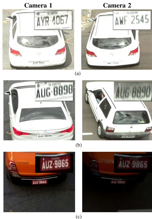
FIGURE 1. Examples of challenging scenarios for vehicle identification: (a) similar vehicles with different license plates; (b) similar license plate strings and distinct vehicles; and (c) same vehicle under different lighting conditions. The combination of attributes, e.g. vehicle appearance and textual information from the license plate region, can help to improve the recognition since two similar vehicles may have considerably different license plates and vice versa.
