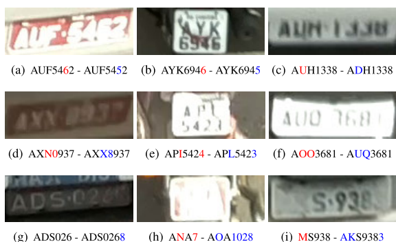
FIGURE 11. Examples of license plates that were partially or not recognized by the CNN-OCR architecture. For each license plate, we show the predicted and ground truth strings, where the red and blue characters denote the CNN-OCR misreadings and the ground truth, respectively.
