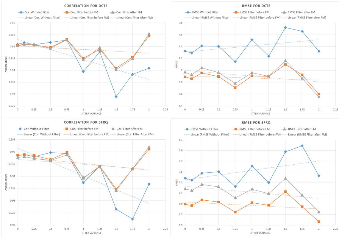
FIGURE 16. Correlation and RMSE using DCTE and SFRQ as FM with different values of variance of Jitter noise \sigma_{\eta}^2 = (2a_2k + a_1)^2\sigma_{\epsilon}^2 + 2a_2^2\sigma_{\xi}^4 ; without using Kalman filter, with filter as pre-FM step and filter as post-FM step. The dotted line shows the linear trend of the data.
