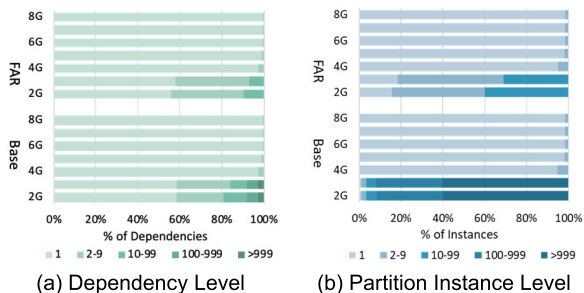
FIGURE 7. Dependency and partition instance histograms for BFS executions with different execution memory allocation.
