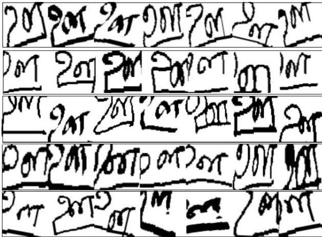
FIGURE 21. Sample augmented images belonging to a character [Row-1: Rotation, Row-2: Horizontal Shift, Row-3: Vertical Shift, Row-4: Zoom, Row-5: Multiple effects].
