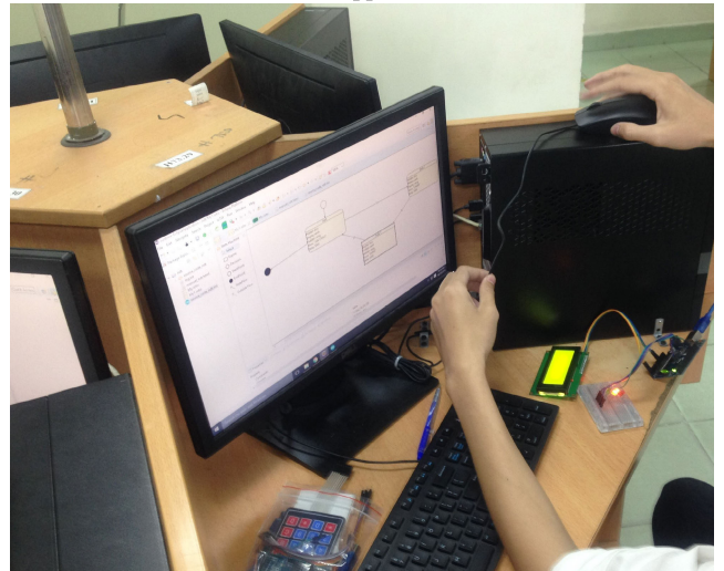
(b) Checking C++ source code that was generated thanks to Micraspis before bootloading.
