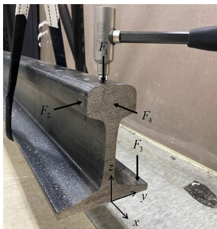
FIGURE 11. Position of impact force excitation on the rail specimen.
