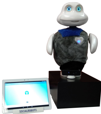
FIGURE 2. Mini, a social robot used to assist older adults with mild cognitive impairment in cognitive stimulation therapies.
