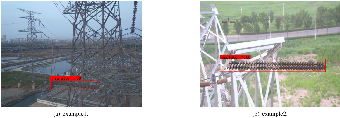
FIGURE 3. The recognition of insulator using deep learning method.
