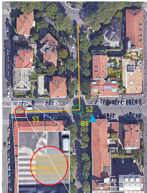
FIGURE 4. Urban scenario used in simulations: the solid yellow line represents the reference vehicle trajectory, the blue triangle the mmW BS (located at 6 m height from ground) while red and green circles the S1 and S2 locations used for testing the proposed LR channel estimation. The inset illustrates the gridding used by the ray-tracing to emulate the multiple vehicle passages by SUMO.
