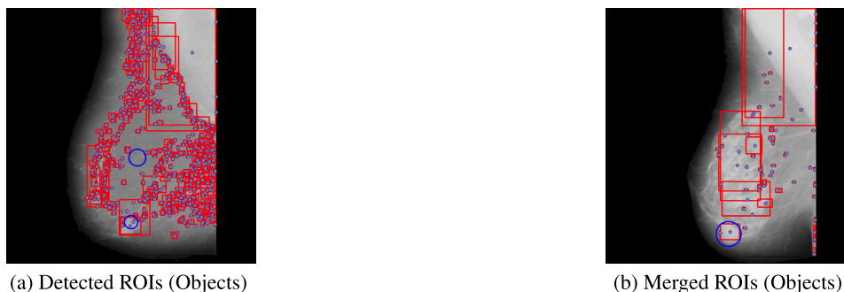
FIGURE 5. The figure shows the intermediate results of detected regions and their merging process in hierarchical clustering.
