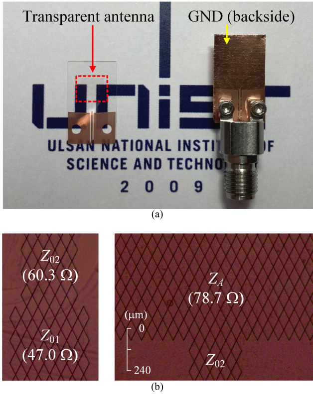
FIGURE 14. Photograph of (a) the fabricated optically transparent antenna and (b) zoomed-in view of antenna structure with the designed characteristic and antenna impedances.
