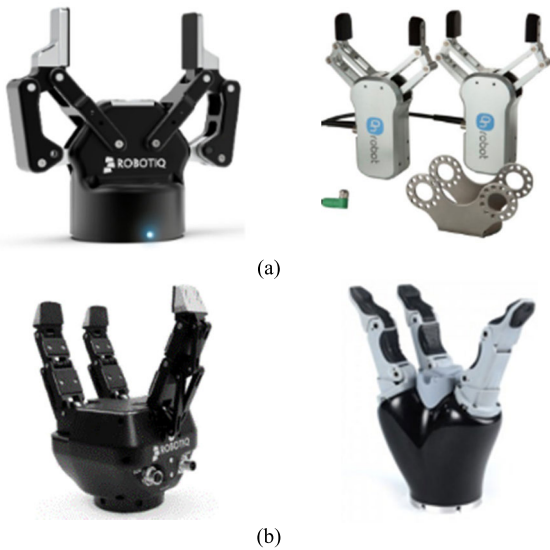
FIGURE 1. Fingered end-effectors: (a) 2-finger type, (b) 3-finger type [3], [4].
